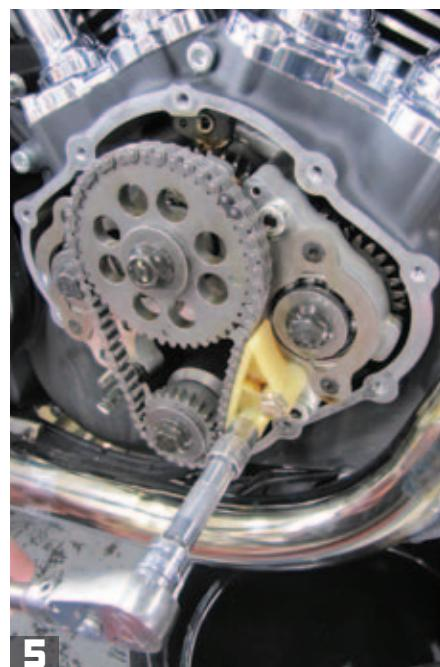
**5** Dan removes the two bolts that hold the chain guide block using a 10mm socket. Then, after noting its orientation, he pulls the chain guide from the camshaft bearing carrier.
