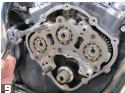
**9** He then uses a 6mm Allen to remove the three remaining cam bearing carrier bolts. Dan now threads just the two exhaust camshaft bolts partway back into their camshafts.
