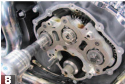
**8** Dan uses a 15mm socket and an impact gun to remove the front and rear exhaust camshaft bolts and their thick washers from the engine.
