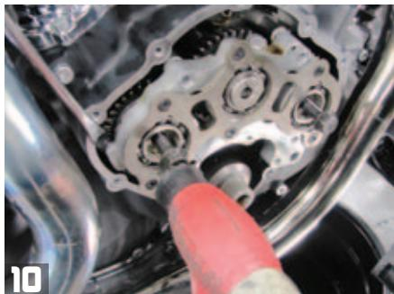
**10** To remove the bearing carrier, Dan gently pries on the carrier's three ears using a flat-bladed screwdriver. If any of the cams start to move out with the carrier, he gently taps them back onto the engine using a plastic mallet. Don't let the cams come out of their bearings in the right crankcase!
