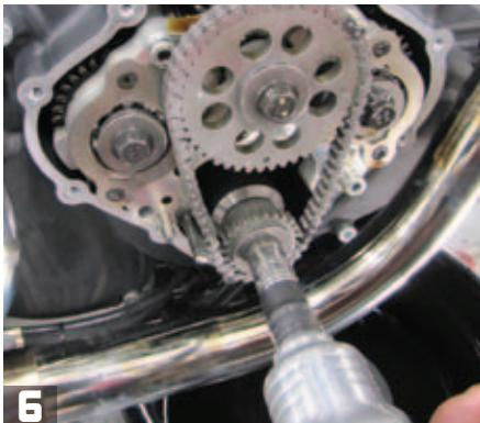
**6** Using a 15mm socket and an impact gun, Dan removes the pinion sprocket bolt and the center intake camshaft sprocket bolt, as well as their thick washers. He then sets them aside for reinstallation later on.
