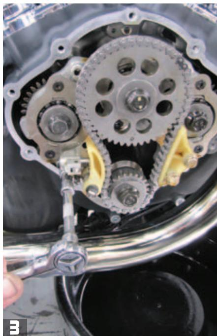
**3** Dan can now start the disassembly. He removes the chain tensioner bolt using a 6mm Allen. After noting its orientation, he pulls the tensioner from the camshaft bearing carrier and sets it aside for reinstallation later.
