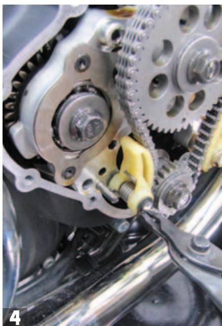
**4** Dan removes the tenstioner shoe retainer circlip using external circlip pliers. Then, after noting how its spring is orientated, he pulls the tenstioner shoe from the camshaft bearing carrier and sets it aside for reinstallation later.
