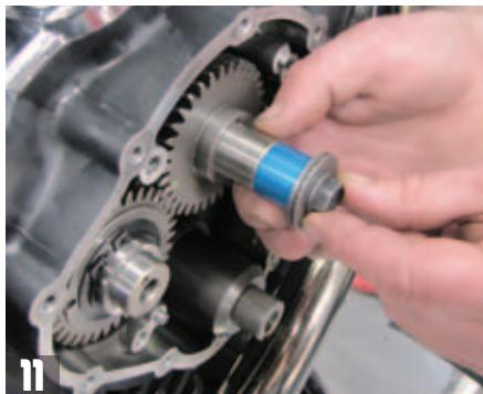
**11** To install the RDS Indian camshaft removal tool, Dan slips the RDS spacer with the hole over the locating pin on the center camshaft and secures it finger-tight using the stock thick spacer and bolt.
