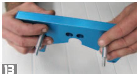
**13** To prepare the RDS tool's body, Dan slips two of the RDS-supplied bolts into the tool. He then slips two of the long RDS spacers over the bolts.
