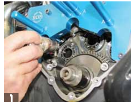
1 With some assembly lube on its inner bearing surface and cam lobe, Dan installs all three of the new camshafts into their bearings in the right crankcase.
