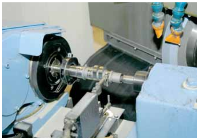
Grinding camshaft journal bearings
