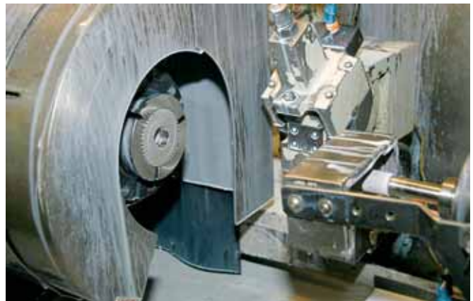
Grinding internal diameters on a programmable ID grinder.
