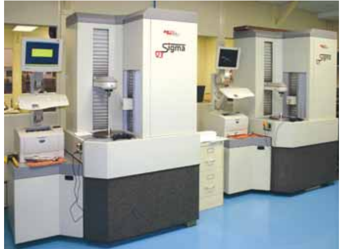
M & M 400 CNC gear inspection systems in temperature controlled room
