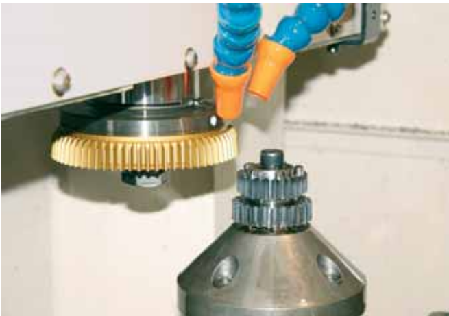
Cutting gear teeth with a Lorenz CNC gear shaper.
