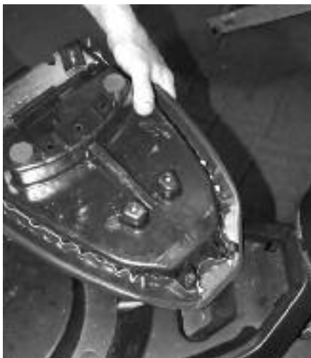
28 The front of the seat has these two clips that engage two slots on the bike. The rear of the seat engages its studs first, then the front of the seat snaps into place. AIM
