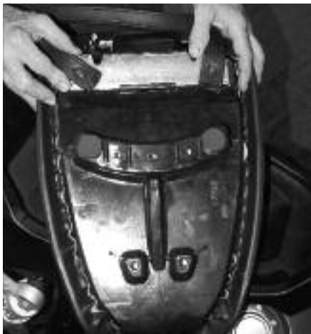
27 After reinstalling the bodywork and before you reinstall the front seat, ensure the passenger strap steel support is fully engaged in its slot in the bottom of the seat.
