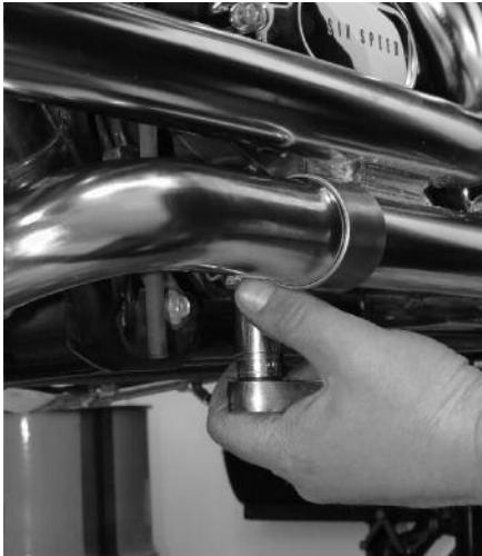
**14** Once he has the clamp hardware inboard of the pipe, Rob uses a 5/8" socket to torque the hardware to 25-30 ft-lbs. He then puts some muffer cement outside the rear end of the rear header.
