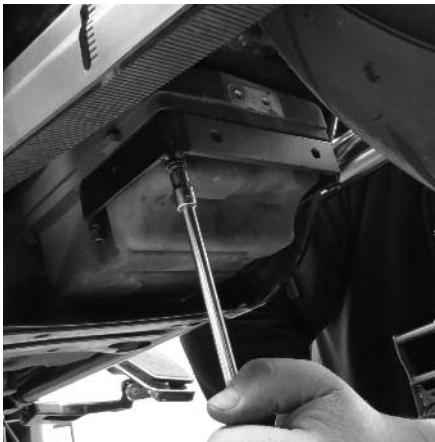
**9** Ron installs the new black S&S-supplied exhaust mounting bracket to the oil pan using the new S&S-supplied bolts, blue Loctite, and a 3/16" Allen. He torques the bolts to 100-120 in-lbs.
