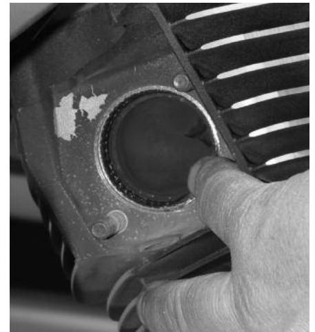
**2** After removing the old exhaust gaskets from the exhaust ports using a pick tool, Rob slips in the new S&S-supplied gaskets with his finger.
