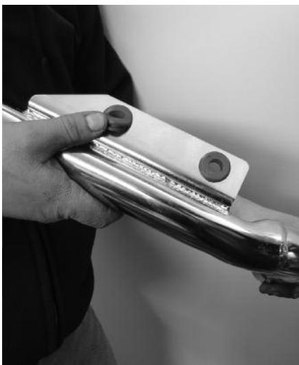
**10** Rob then slips the S&S-supplied red rubber grommets into the S&S-supplied front cylinder crossover pipe mounting bracket using just his fingers.
