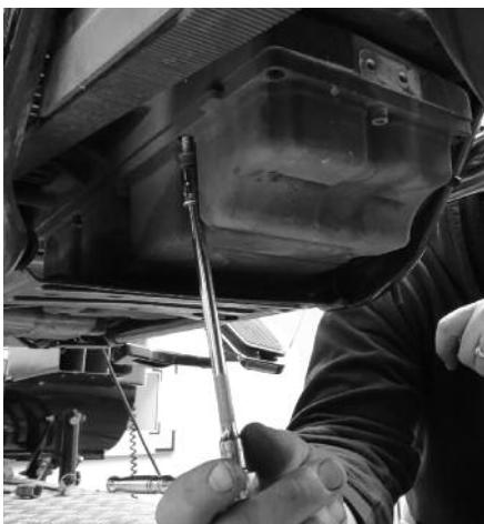
**8** He then uses a 3/16" Allen to remove these four bolts from the oil pan, so he can mount the new S&S exhaust mounting bracket.
