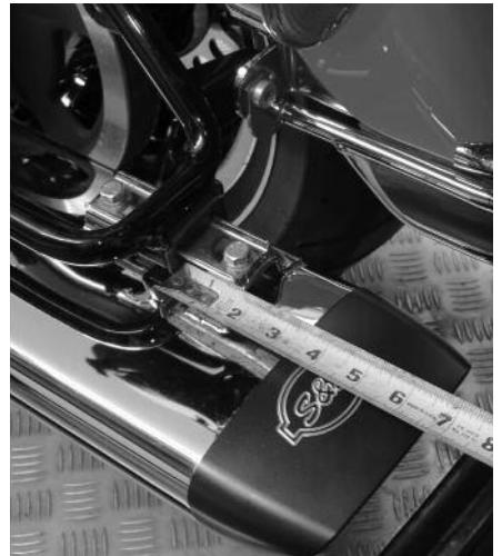
**18** After installing the left muffer in the same way, Rob uses a ruler to ensure both mufflers are protruding the same distance from their mounting bracket.
