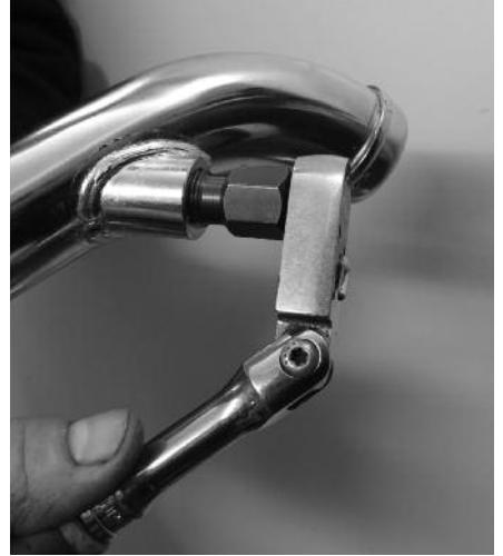
**3** Rob always sends an 18mm-1.5 tap through a new exhaust header's O<sub>2</sub> sensor ports to ensure the threads are clear. These were fine.
