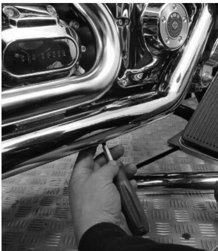
**20** After wiping down the entire system with glass cleaner, Rob installs the front heat shield using a 1/4" socket or flat-bladed screwdriver. He torques the clamp to 20-40 in-lbs.
