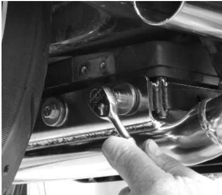
**13** Rob slips the crossover pipe over the S&S header's front cylinder pipe and secures it to the bracket using the S&S-supplied hardware, blue Loctite, and a 1/2" socket.
