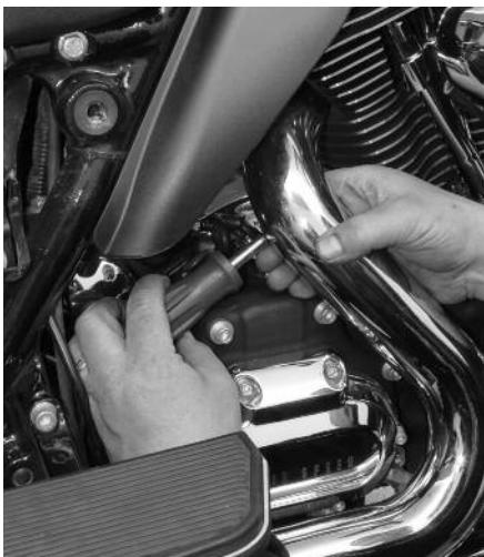
**21** Yup, Rob installs the rear heat shield in the same way using a 1/4" socket or flat-bladed screwdriver. He then wipes down both heat shields with glass cleaner.
