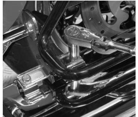
**16** After he puts muffer cement inside the forward end of the muffer, Rob slips the muffer over the pipe and secures the muffer to the stock mount using the stock hardware, blue Loctite, and a 9/16" socket.
