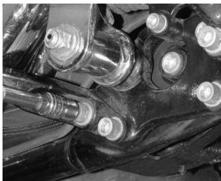
**22** Rob reconnects the right floorboard using some blue Loctite, the stock hardware, and a 5/16" Allen. He also pops the right side cover back onto the bike.
