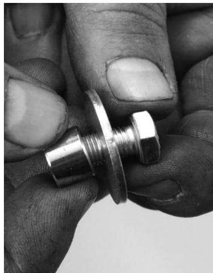
**12** Rob slips a S&S-supplied large washer and spacer over each of the two S&S-supplied bracket mounting bolts. He then puts some muffler cement on the outside of the front cylinder header.
