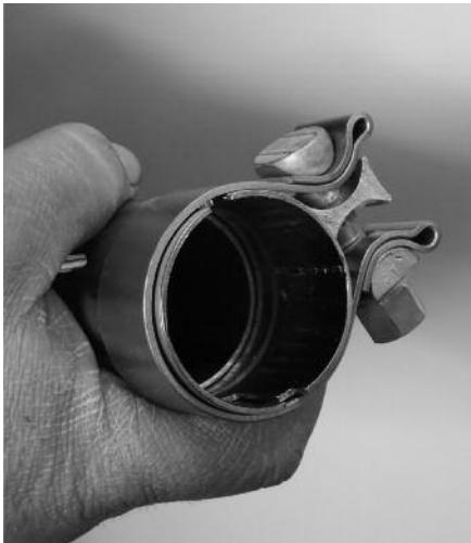
**15** Rob now slips a new H-D muffer clamp over the forward end of the S&S right muffer (no, they're not the same), so the hardware will be facing in toward the bike.
