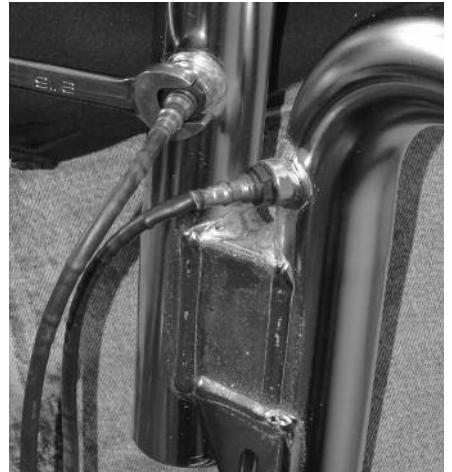
**4** After putting a little anti-seize on the threads (don't get any on the sensor bulbs), Rob installs the stock O<sub>2</sub> sensors in the new S&S header using a 9/16" wrench. He torques them to 30-44 ft-lbs.
