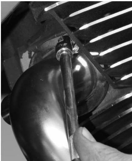
**6** He installs the S&S header onto the engine using new H-D nuts and a 1/2" socket. He leaves the nuts loose for now, but will torque them to 100-120 in-lbs. once the entire exhaust system is on.
