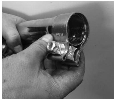
**11** He can now slip the S&S-supplied pipe clamp over the forward end of the crossover pipe. He then puts some muffler cement inside the same end of the crossover pipe.
