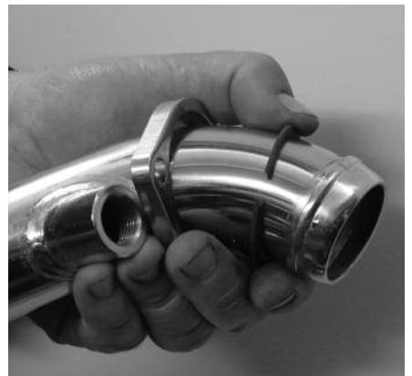
**5** Rob swaps the stock exhaust flanges, with new H-D retaining rings, over to the new S&S header. He then closes off the unused O<sub>2</sub> sensor bungs near them using the S&S-supplied plugs and a 10mm Allen.
