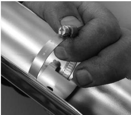
**19** Rob now slips the S&S-supplied clamps inside the S&S chrome header heat shields, so he'll have easy access to their heads once the shields are on the bike.
