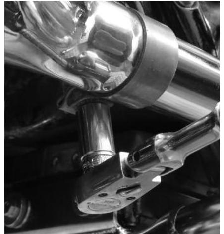
**17** Once he has the clamp hardware inboard of the muffer, Rob uses a 9/16" socket to torque the hardware to 25 ft-lbs. He then torques the exhaust flange nuts to 100-120 in-lbs. using a 1/2" socket.
