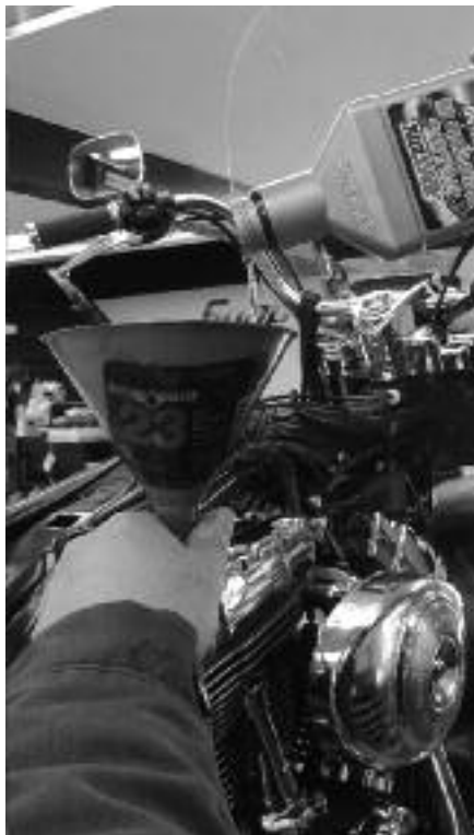
17 Before we hit the dyno to retune the engine, Dan removes the old oil and filter. He then refills the engine with 4 quarts of Amsoil and screws on a new H-D filter.
