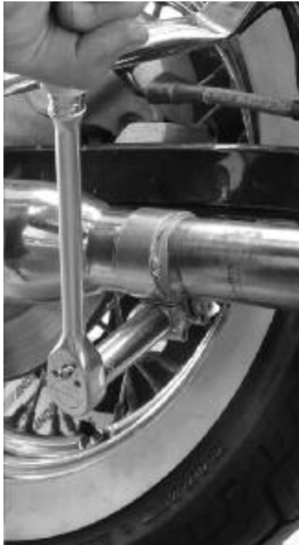
16 Dan insists on using new H-D clamps on the Y-pipe and mufflers to prevent leaks. He also coats the joints with high-temperature muffler cement for the same reason.
