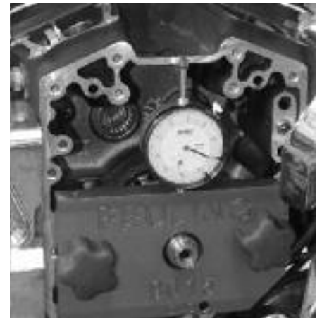
2 Dan first checks the pinion shaft runout using a dial indicator. Ours is 0.0025". Dan also checked the pinion shaft bushing in the support plate and oil pump for excessive wear — none found.
