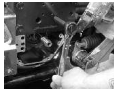
3 Dan then changes the inner cam bearings using a JIMS puller and installer. Dan prefers to use Screamin' Eagle (SE) bearings.
