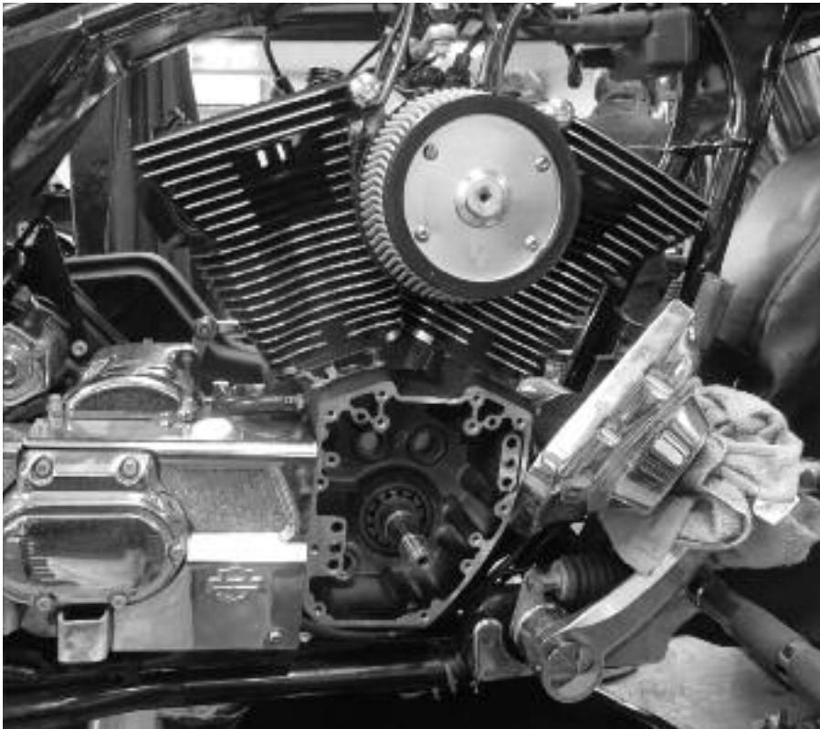
2 Dan first checks the pinion shaft runout using a dial indicator. Ours is 0.0025". Dan also checked the pinion shaft bushing in the support plate and oil pump for excessive wear — none found.
