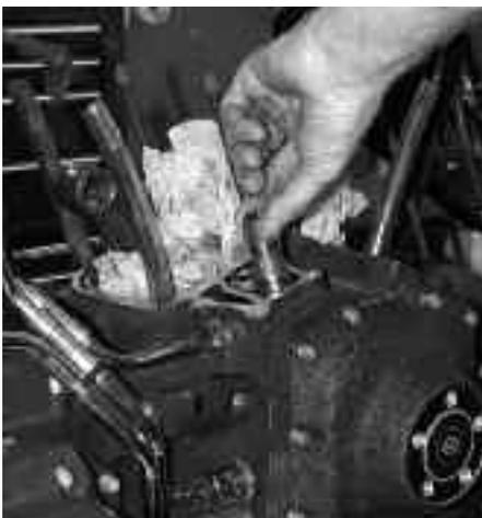
**16** After lubing the rollers on the new H-D lifters, Dirk slips them into their bores in the right case as per their proper orientation.
