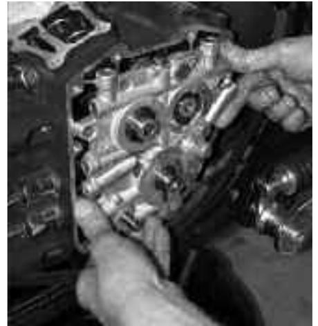
**9** After lubing the inboard ends of both cams, as well as the outboard cam bearings, Dirk slips the cam support plate assembly into the right case. He then checks the cam alignment dots again.
