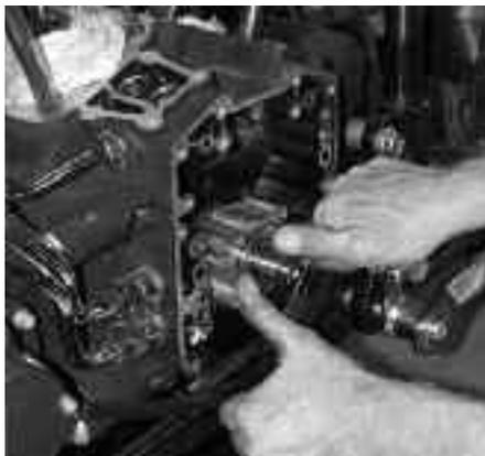
**8** After inspecting the stock oil pump, changing the body O-ring, and lubing its internals, Dirk reinstalls the pump back into the case and on the pinion shaft with a new Cometic O-ring on the pickup tube.
