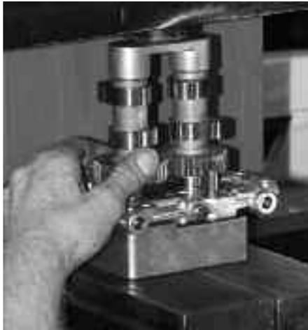
**6** He then uses a special tool and the hydraulic press to press the cams into the plate at the same time. He then rechecks the timing marks to ensure they are still aligned.
