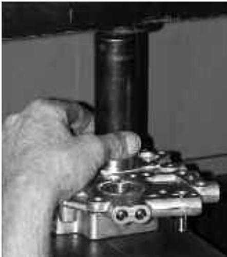
**4** Dirk installs the two new Andrews outer cam ball bearings into the plate using a hydraulic press and the two-piece special tool that supports the cam plate and drives in the bearing.
