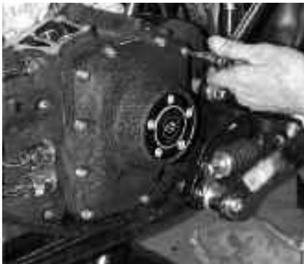
**15** With a new Andrews gasket on the case, Dirk installs the cam cover using the stock bolts, blue Permatex, and a 3/16" Allen. The bolts get torqued to 90-120 in-lbs. as per the H-D procedure.
