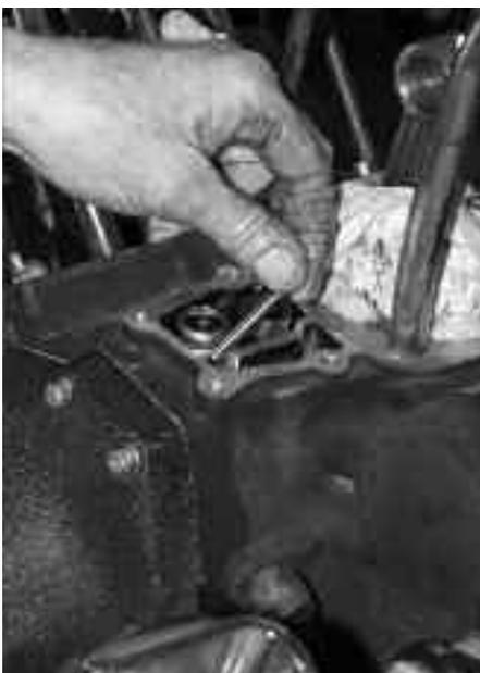
**17** The stock alignment pins go in next, one per lifter set.
