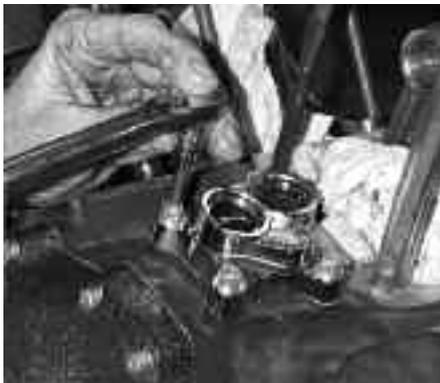
**18** With a new Andrews gasket on the case, Dirk installs the lifter covers using the stock bolts, blue Permatex, and a 3/16" Allen. The bolts get torqued to 90-120 in-lbs.
