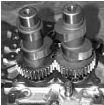
**5** After marking the timing dots, so they are easier to see, Dirk positions both cams in the support plate (the rear one protrudes from the cam cover) and aligns the timing marks.
