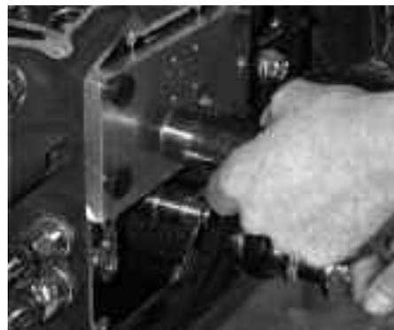
**2** The first step is to take out the stock inner cam bearings and replace them with new Torrington bearings sent with the Andrews cam kit using a bearing removal and installation tool.
