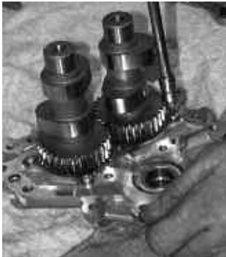
**7** The stock bearing retaining plate is then reinstalled using the stock hardware, some blue Permatex, and a T-20 Torx. These four screws get torqued to 30 in-lbs.
