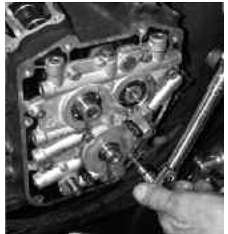
**11** After aligning the pump to the pinion shaft using two alignment pins, Dirk secures the pump using blue Permatex and the stock bolts. He uses a 3/16" Allen to torque them to 90-120 in-lbs.
