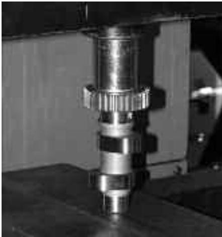
**3** After placing a supplied key on the camshaft, Dirk uses a hydraulic press to install the gear onto the Andrews camshaft. He does both cams in the same way.
