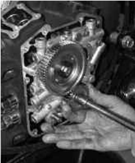
**13** After aligning the timing marks, Dirk installs the pinion drive gear using the Andrews bolt and washer, red Permatex, and a 1/2" socket. This bolt gets torqued to 25 ft-lbs.
