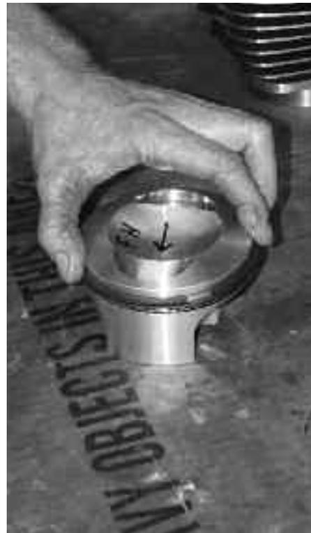
**21** Dirk then installs the piston rings onto the pistons as per the piston manufacturer's instructions regarding dots and bevels for orientation and end gap locations. AIM
