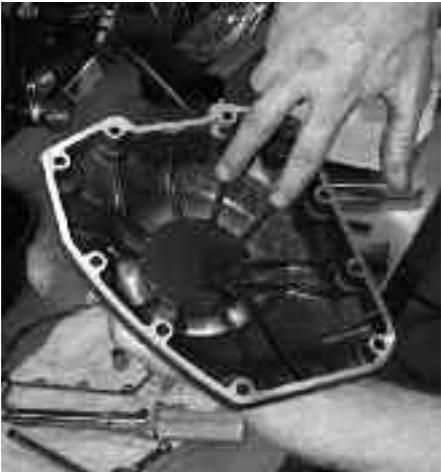
**14** After checking gear backlash as per the Andrews instructions, the cam cover is installed, and the clearance between the rear cam gear and this section of the cam cover is checked.
