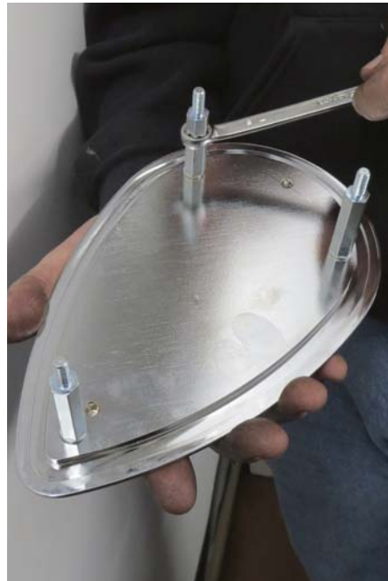
15 Rob installs all three standoffs onto the K&N chrome outer cover using a 7/16" wrench. He torques the standoffs to 100 in-lbs.
