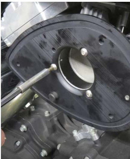
13 Rob installs the base plate onto the crankcase breather plate using a 3/16" Allen and torques the bolts to 100 in-lbs.
