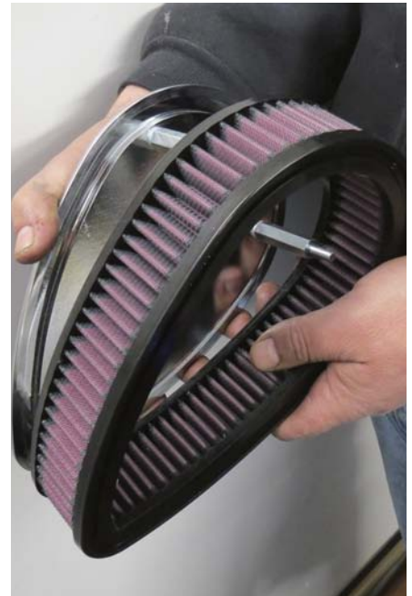
16 Rob positions the K&N filter element onto the chrome outer cover and around the three standoffs.
