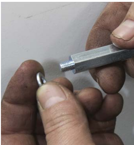
14 Rob then slips the three K&N-supplied lock washers onto the three K&N-supplied standoffs and puts some K&N-supplied blue Loctite on the threads.
