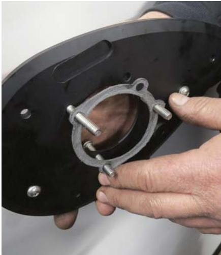
12 Rob then slips the K&N-supplied gasket, orientated as shown, over the three bolts.
