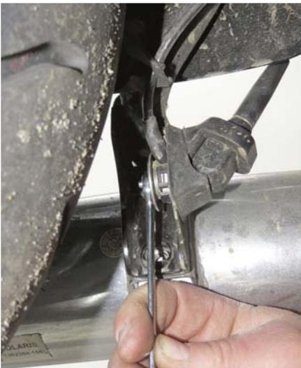
**5** After popping off the rubber cover, Rob uses an 8mm wrench to remove the antenna. He then lays the antenna safely aside for now.
