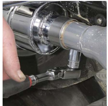
**10** After positioning the clamp vertically (nut facing down) on the muffler, Rob torques the new V&H-supplied Torca clamp to 40-45 ft.-lbs. using a 15mm deep socket.
