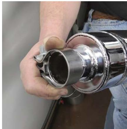
**8** Rob slips the Vance & Hines Torca muffler clamp onto the front of the right V&H muffler. He then coats the inside of the muffler with muffler sealant, as he does with all his exhaust installs.
