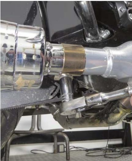
**4** Rob uses a 15mm deep socket to loosen the right muffler's header clamp.
