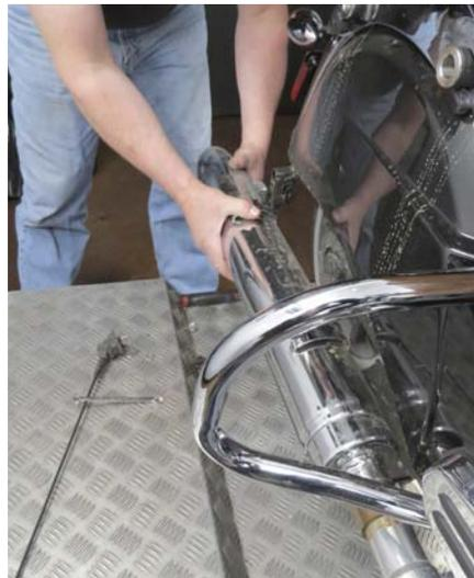
**7** Rob gently moves the muffler slightly up and down as he pulls it back to get it off its header pipe.
