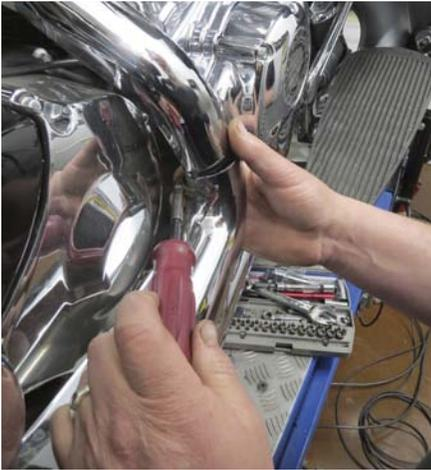
**3** Using a 1/4" nutdriver, Rob opens the stock rear heat shield front clamp. You can also use a flat-bladed screwdriver.
