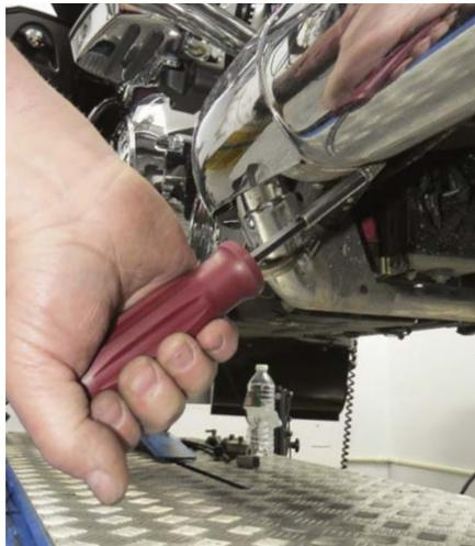
**13** Uses a 1/4" nutdriver, Rob opens the stock left heat shield clamps and does the same for the left muffler as he did for the right, but without the antenna.
