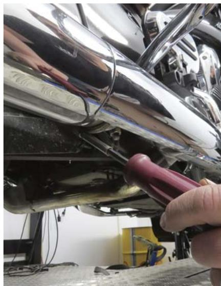
**2** Using a 1/4" nutdriver, Rob opens the stock rear heat shield rear clamp. You can also use a flat-bladed screwdriver.
