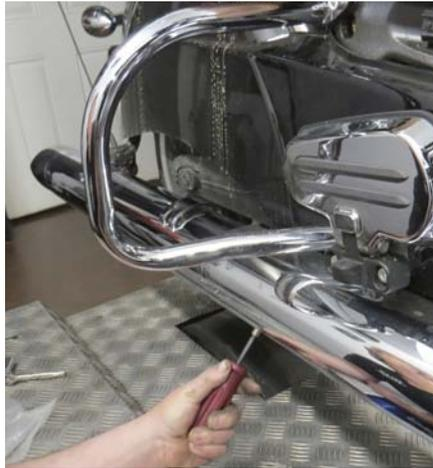
**12** Rob then reinstalls the stock heat shields using a 1/4" nutdriver. You can also use a flat-bladed screwdriver.
