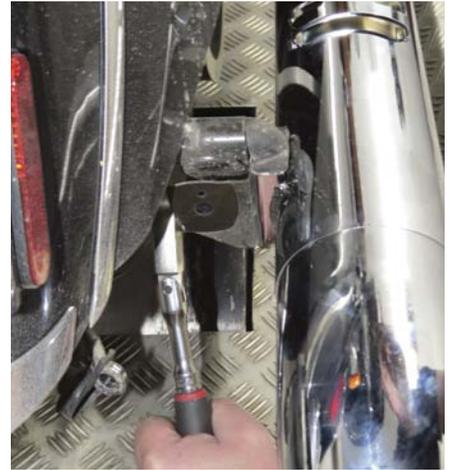
**9** After slipping the new V&H muffler onto the stock header, Rob attaches the new muffler to the stock bracket using the V&H-supplied flanged bolts, blue Loctite, and a 1/2" socket.
