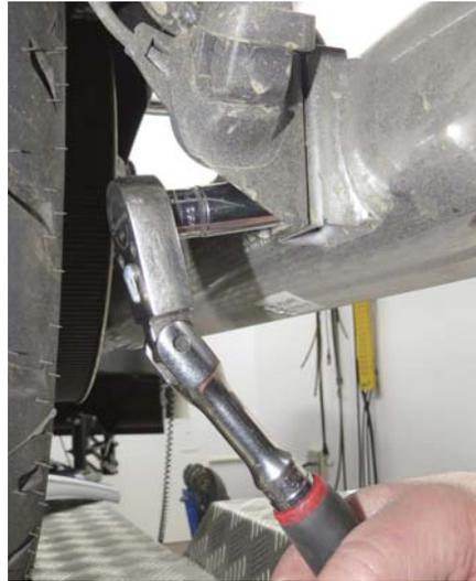
**6** Rob can now use a 13mm deep socket to remove both rear right muffler support bolts.
