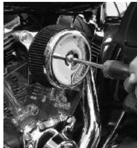
11 The Boyesen chrome outer cover is installed using a #3 Phillips screwdriver and the Boyesen-supplied bolt. You can also use the stock air cleaner cover if you want.
