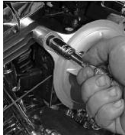
9 The two breather bolts are now torqued to 14 ft.-lbs. using a 9/16" socket. Then remove the 2-3/4"-long bolt installed earlier in the bottom hole.
