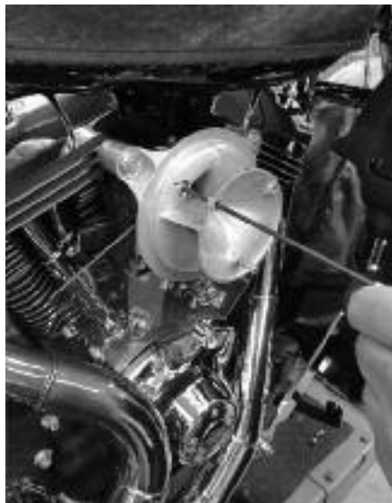
8 Bolt the X-Intake to the throttle body using the two Boyesen-supplied 1"-long screws and a 5/32" Allen. Torque the screws to 10 ft.-lbs.
