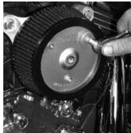
10 Secure the Boyesen element onto the X-Intake using the two Boyesen 3/8"-long bolts in the two upper holes and the 2-3/4" bolt in the lower hole. Torque the bolts to 10 ft.-lbs. using a 3/16" Allen.
