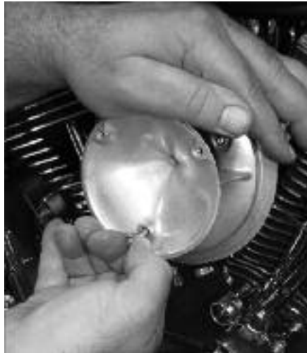
6 Insert the Boyesen-supplied 2-3/4" screw into the bottom hole of the X-Intake and loosely secure the X-Intake to the throttle body.
