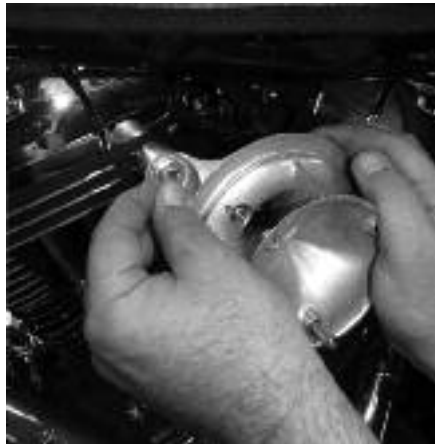
7 After putting some blue Loctite onto the Boyesen-supplied breather bolts, loosely secure the X-Intake assembly to the heads.
