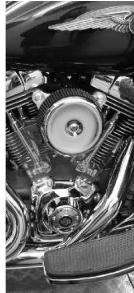
12 Here's how the finished Boyesen Power X-Intake looks on our 2013 Ultra Limited.
