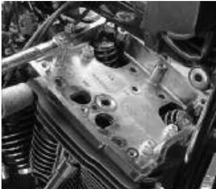
**20** With new Cometec gaskets and O-rings on each head, Dan installs the stock lower rocker boxes using the stock bolts, blue Loctite, and a 7/16" socket. He torques the bolts to 150 in-lbs. as per the H-D procedure.
