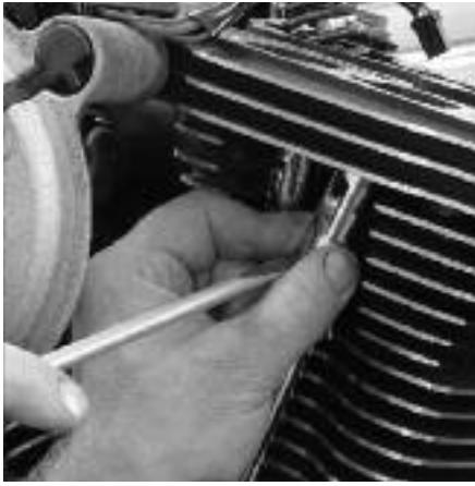
**19** After Dan installs new Cometec O-rings into both heads, all four lifter covers, and all four stock pushrod tubes, he installs the pushrod tubes onto the engine and pops in the top clips using a flat-bladed screwdriver.
