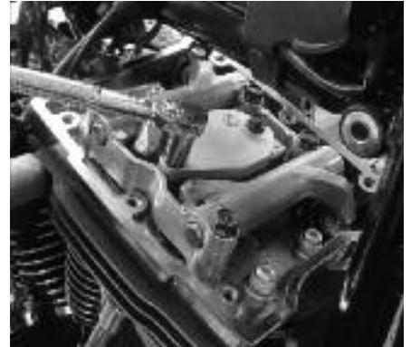
**24** While the lifters are bleeding down, Dan torques the breather bolts to 120 in-lbs. using a 3/8" socket. Once he can spin the pushrods with his fingers, Dan does the same on the other head.
