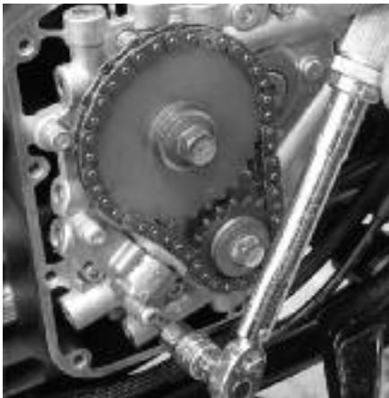
**14** Dan installs the stock outer hydraulic chain tensioner using the stock bolts, blue Loctite, and a T-27 Torx. He then torques the bolts to 90-120 in-lbs.
