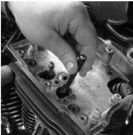
**21** After spraying brake cleaner through the oil hole in each stock pushrod and letting it air dry, Dan drops the long black exhaust pushrods and short silver intake ones into their respective pushrod tubes through the boxes.
