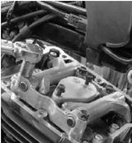
**23** With this head's lifters at their lowest points, Dan installs the stock rocker assembly using the stock bolts, blue Loctite, and a 1/2" socket. He torques the bolts to 15-18 ft-lbs. in a crisscross pattern.
