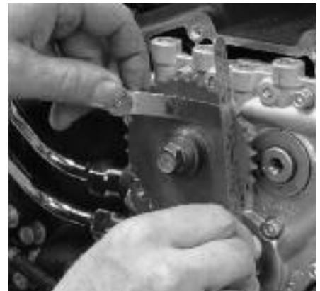
**11** With the stock 0.120" spacer on the rear cam, Dan installs both stock sprockets. He then checks the sprocket alignment using a steel straightedge and a flat feeler gauge. The gap between them must be and is under 0.010". He then removes both sprockets.
