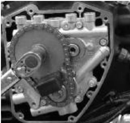
**13** Dan installs the stock sprocket bolts and washers onto the engine using a SE locking tool, red Loctite, a 1/2" socket, and a 9/16" socket. He torques the bolts to 25 and 35 ft-lbs. respectively, as per the H-D procedure.
