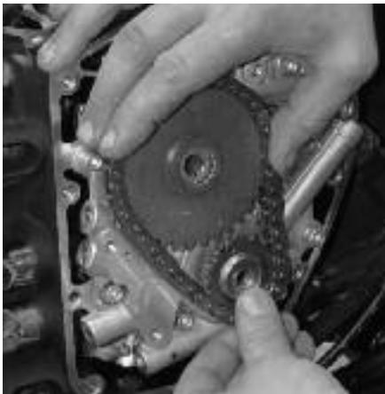
**12** With the pinion sprocket dot aligned with the line on the support plate, Dan wraps the stock outer chain around both sprockets (noting their alignment dots). He then slips both sprockets onto their respective shafts.
