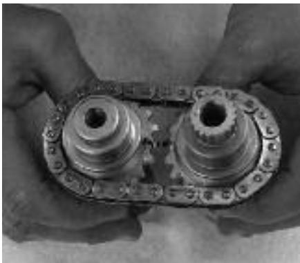
**5** Dan then wraps the stock inner cam chain around the new Lunati cams noting their timing marks and the mark he made on one side of the chain before he removed it.
