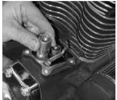
**16** After Dan pumps up each of the four new Lunati lifters with fresh engine oil, he drops them into their bores in the right case with one of their flat sides against where the alignment pin will rest.
