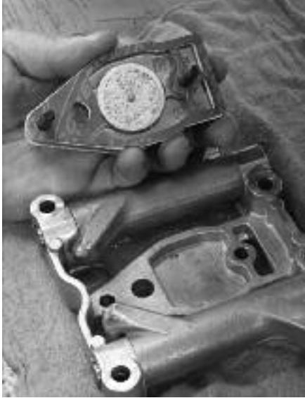
**22** After Dan replaces the foam filter elements, umbrella valves, and gaskets in both stock oil breathers, he positions each breather onto its rocker arm assembly support complete with both its bolts.
