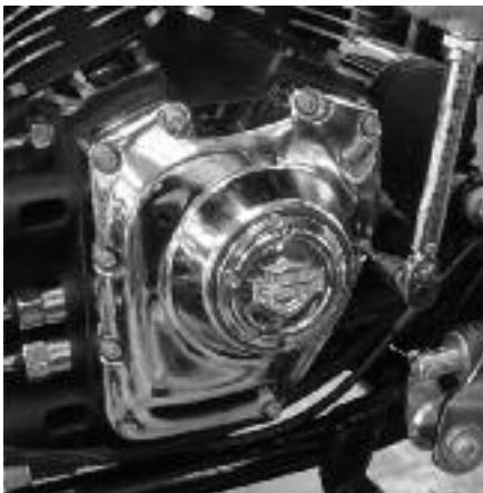
**15** With a new Cometic gasket in place, Dan installs the stock cam cover using the stock bolts, blue Loctite, and a 3/16" Allen. He torques the bolts to 90-120 in-lbs. as per the H-D procedure.
