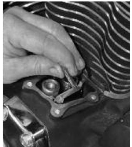
**17** The alignment pin is the next part in. Dan then cleans off any oil that dripped onto the lifter cover gasket surface and positions a new Cometic gasket onto each lifter cover base.
