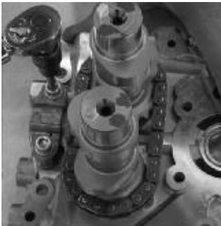
**8** Dan installs the stock inner chain tensioner using the stock bolts, blue Loctite, and a 3/16" Allen. After he torques the bolts to 90-120 in-lbs., he puts lube on the cam lobes, chain, and inner cam bearing surfaces.
