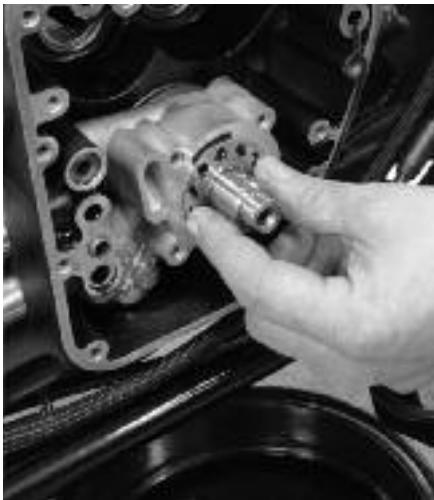
**4** Once he has slipped new Cometic O-rings onto the oil pump and right case, Dan assembles the stock oil pump in the gearcase compartment using lots of assembly lube on all the gerotor gears.
