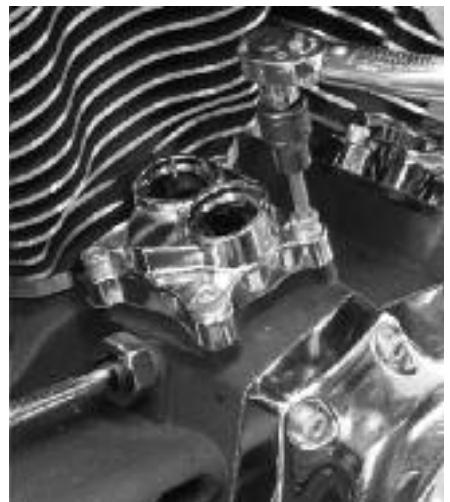
**18** Dan reinstalls the stock lifter covers onto the right case using the stock bolts, blue Loctite, and a 3/16" Allen. He torques the bolts to 90-120 in-lbs. in a crisscross pattern.
