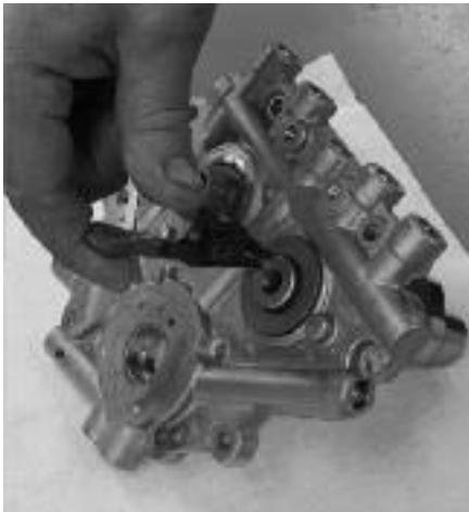
**7** After Dan slips the stock 0.100"-thick spacer over the end of the front cam, he secures it using a new H-D retaining ring and external snap ring pliers. He then rotates the retaining ring to ensure it's fully in its groove.
