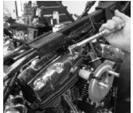
**25** With a new Cometec gasket on both bottom boxes, Dan reinstalls the stock covers using the stock bolts (long ones on the pushrod side), blue Loctite, and a 7/16" socket. He torques the bolts to 150 in-lbs. in a criss-cross pattern.
