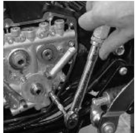
**10** Dan aligns the oil pump by spinning the engine and using two JIMS alignment dowels. Once he has finished the procedure outlined in Tips & Tricks, he torques all four stock bolts to 90-120 in-lbs.
