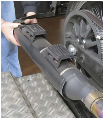
5 After spraying some AeroKroil in the seam, Rob pulls the right muffer from its header pipe by gently rocking it up and down, and side to side while pulling it back from its header pipe.
