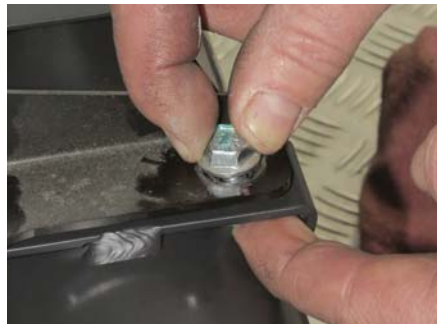
8 Rob slips the Bassani-supplied bolts, with some blue Loctite on them, through the bracket and puts a Bassani-supplied nut onto each bolt. He just snugs the hardware for now using a 13mm wrench and 13mm socket.
