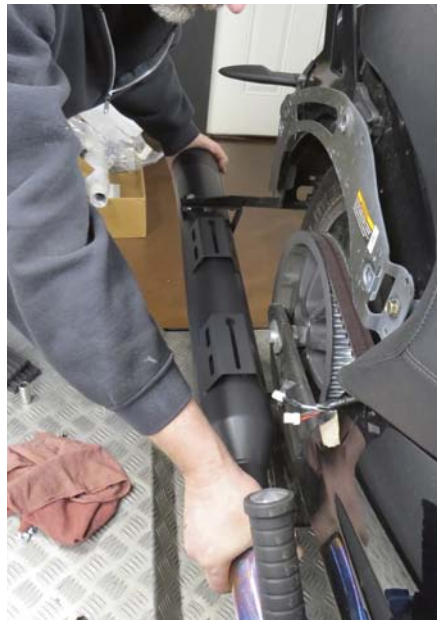
7 Rob then installs the new Bassani muffer onto its header pipe by gently rocking it side to side until the rear mounting holes are aligned.
