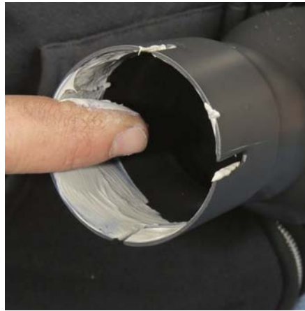
6 Rob puts some Yale Automotive muffer cement inside the front opening of the new Bassani right muffer and then slips a new Victory muffer clamp (#7081340/$20.99) onto the muffer with its hardware to the inside.
