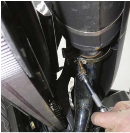
3 Rob uses a 15mm socket and some AeroKroil to open up the muffer clamp. He then pulls the heat shield from the right muffer.
