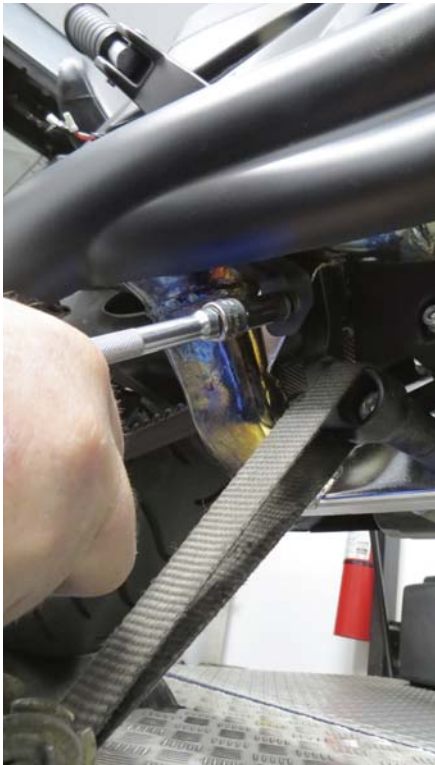
12 Rob now reinstalls the stock muffer heat shield using a 10mm socket on the front stock bolt and a 3/8" nutdriver on the rear clamp. Rob then does the same on the left muffer system.
