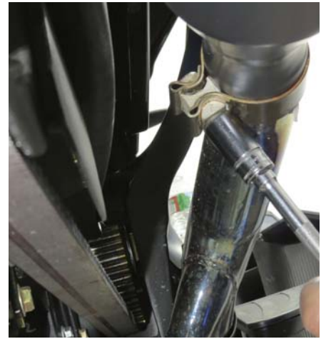
9 With the front muffer clamp aligned with the edge of the muffer, Rob torques the clamp to 35-40 ft.-lbs. using a 15mm socket.
