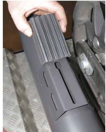
11 After pulling the stock rubber saddlebag insulation pads from the stock right muffer, Rob slips them onto the new Bassani right muffer.
