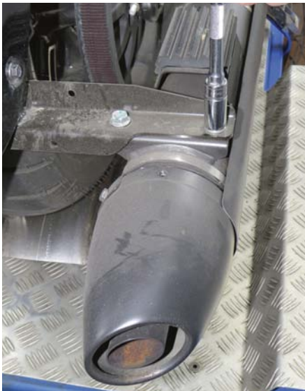
4 Rob uses a 13mm socket to remove the two rear right muffer support bolts.
